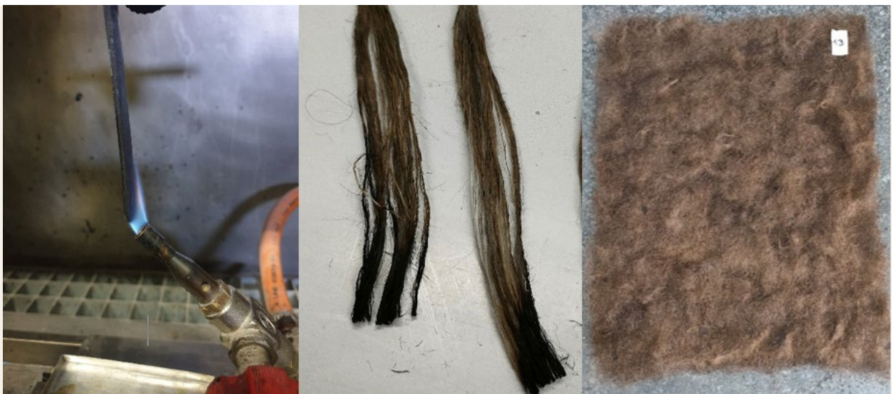
PA-11 with FR, flax fiber with FR and jute fiber functionalized.
